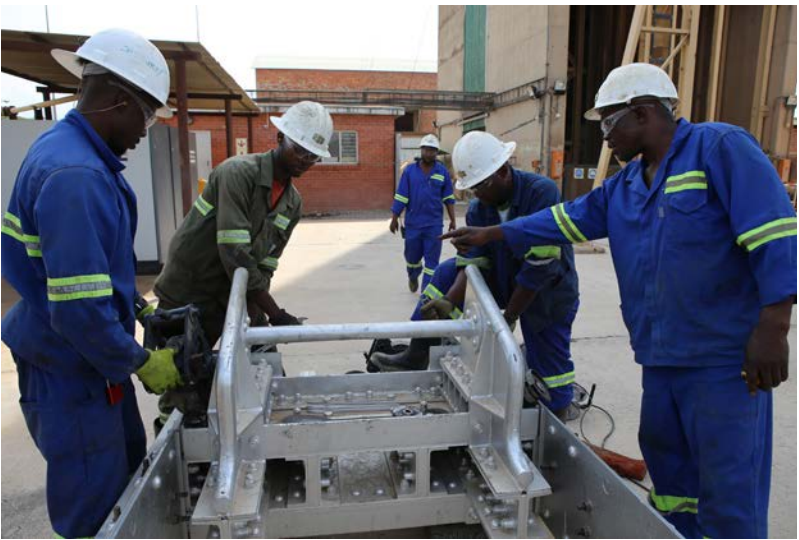
Skip assembly at the shaft (installation of cluster frames on the bridge)
